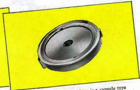
Transmitter —The transmitter is a capsule type of feltless construction redesigned for improved acoustic control. A shield-protected one-piece phosphorus bronze diaphragm and gold electrodes make this new transmitter most reliable under adverse humidity and temperature conditions. It has greater electrical output, good non-positional qualities, and excellent response throughout a wide range of applied voltages.
