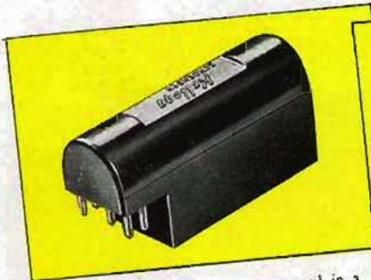
Condenser —A single condenser encased in a molded bakelite housing is standard for all types of subscribers' services. Electrical terminations are pin plug type; condenser plugs into the pin jacks located on the Interconnecting Block. The capacity control switch (see item 2, page 5) varies condenser capacities to 0.5 or 1.0 microfarad as required for the various ringing applications.
