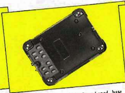
Base Plate —The rectangular shaped base plate is 3 x 7 inches, drawn from heavy brass, finished in black. Modern chemical treatment affords scratch protection while cutting down corrosion vulnerability. Sound openings are screened against dust and insects.
