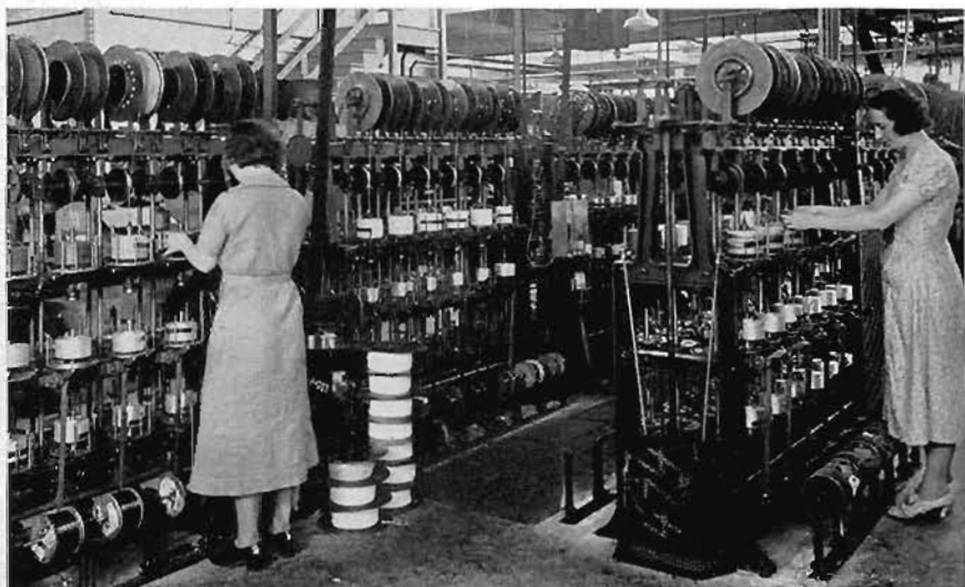
90 MILES A DAY! This is the kind of speed at which these machines insulate wire and finzel. Each machine of this group applies up to 3 coverings of silk or cotton to 6 different conductors AT THE SAME TIME! Only purified silk and long-fibre cotton of the highest grade are used.
