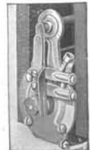
Pulsating & Alternating Current Generator Terminals
