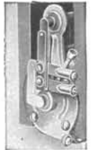
Alternating Current Generator Terminals
