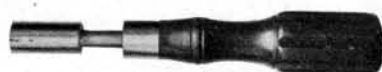
Fig. 262 Socket Wrench for Nuts on Nos. 16 and 22 Binding Posts. Also for Nuts on Ringer Gongs. Pc. 6462.
