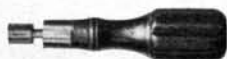
Fig. 263 Socket Wrench for Relay Armature Nuts. Pc. 11039. Also for Standard Arrester Nuts. Pc. 3098.
