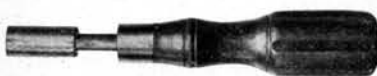
Fig. 261 Wrench for 77 Nut. Used for removing major relays from the mounting strip. Pc. 3095.
